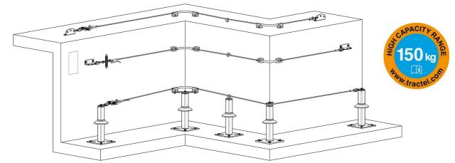
The Travspring<sup>™</sup> One single-cable system is a proximity and sporadic use lifeline. It requires a double lanyard to cross the intermediate and corner anchors.
